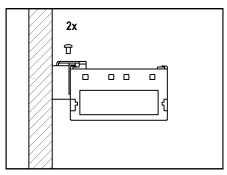
Level fixture prior to final tightening of hardware.
