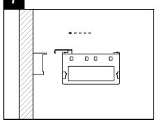
With 2 people, raise fixture into position and engage it on hooks located on top of wall brackets. Secure bracket using supplied hardware.
