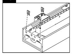
Slide spring clips onto existing wall mounted fixture.
