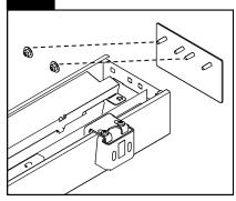
Attach endcap to first and last module in each row using supplied hardware. Use the two endcap studs shown in above image.
