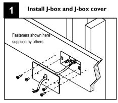
Determine power feed location and install 2"x4" J-box (supplied by others) parallel with the fixture. Complete connections at J-box with supplied power cord. On supplied J-box cover plate, feed power cord through rectangular hole. Secure cover to wall and J-box using applicable hardware (supplied by others).
