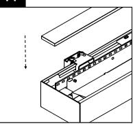
Locate LIGHTGUIDE panel in fixture box, peel protective layer from both sides of panel, and install **SHINY SIDE DOWN** in fixture as shown.
