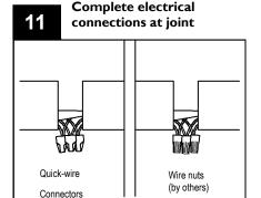
**NON-POWER LOCATIONS:** Use supplied quick-wire connectors. Tuck wires into wire cavity.
