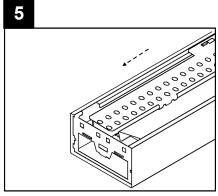
Remove TOP REFLECTOR by sliding to one side then lifting off.
