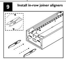
For each additional fixture in the row, at the end where it will join to the existing wall mounted fixture, insert joiner aligners into the crossplate (aligners will lock into place).
