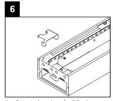
Install required number of rail brackets, per steps 2-3, on the housing. Slide along the length of housing to approximate location matching the brackets on the wall.
