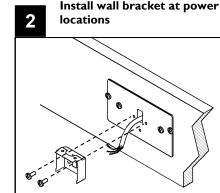
**RECOMMENDED:** Feed power cord through top of wall bracket and attach to J-box cover with 2 screws (supplied). Leave power cord outside wall for connection.
