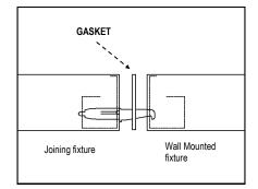
With two people, raise second fixture to wall. At joint, insert joiner aligners through black **GASKET** and into wall mounted fixture. At other end of joining fixture, install wall bracket as in step 7.
