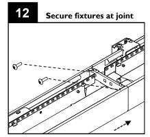
Slide second fixture flush against first fixture. Secure joint using supplied hardware. Secure and level fixture to wall bracket as in step 7. For additional fixtures, repeat steps 9-12.
