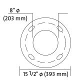
Bolt circle 12-1/2" (318mm) Mounting details Comes with 4 steel anchor bolts, 5/8" x 12", 4 nuts and 4 washers. Important: Do not obstruct space between anchor
