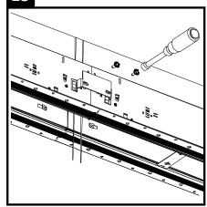
Install joiner brackets on each side of the housing using supplied hardware. Important: Hand tighten bracket screws while supporting the housing on the opposite side. Gradually alternate sides while tightening.
