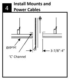
Install a 'C' channel perimeter around the ceiling cutout.
