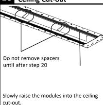
Important: For continuous row modules, start at one end and gradually raise each module up one inch at a time. Repeat process until housing is fully recessed and housing trim touches drywall ceiling. Do not stress the joint connection by tilting the module, as damage can occur.
