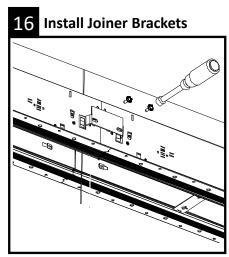
Install joiner brackets on each side of the housing using supplied hardware. Important: Hand tighten bracket screws while supporting the housing on the opposite side. Gradually alternate sides while tightening. Do not over tighten.
