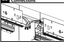
Complete module to module wiring connections and carefully tuck all wires inside the upper wiring cavity.
