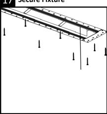
Secure the fixture to the gyproc and 'C' channel with #6 drywall screws (supplied by others)
