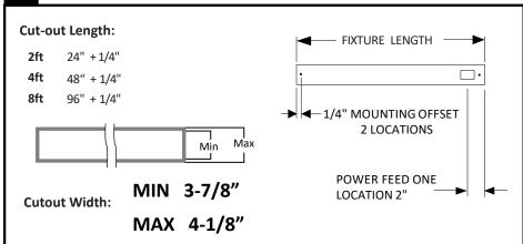
Important: For 2ft standalone fixtures, end framing members must be installed 1" beyond ceiling cut-out.
