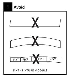
The straightness and accuracy of the cut-out in the drywall is crucial in ensuring proper fit for the fixture.
