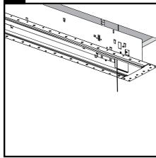
Once the power connections are complete, pull the aircraft cable to raise all modules to just below the ceiling.
