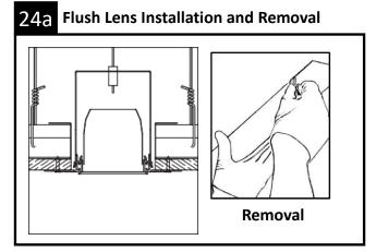
Flush Lens: Snap in lens into fixture. Lens Removal: To remove snap-in lens for maintenance purposes, insert a flat, smooth edged object between lens and housing. Twist to release pressure and remove lens.
