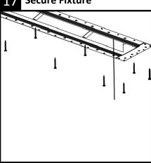
Secure the fixture to the gyproc and 'C' channel with #6 drywall screws (supplied by others).
