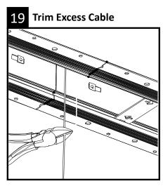
Trim suspension cable approximately 8 inches below the ceiling level. Tuck all excess cable inside the upper wiring cavity.
