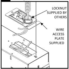
At the power location(s), remove factory installed wire cover. Feed power wires through. Complete all wiring connections.
