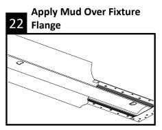
Mud over the fixture flange. When finished, use a utility knife to cut out the mud guard.
