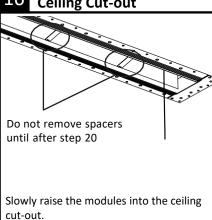
Important: For continuous row modules, start at one end and gradually raise each module up one inch at a time. Repeat process until housing is fully recessed and housing trim touches drywall ceiling. Do not stress the joint connection by tilting the module, as damage can occur.
