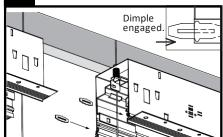
At joint location(s), gently tap provided joiner aligners inside one module only. Two joiner aligners are required for each joint.
