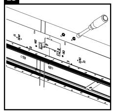
Install joiner brackets on each side of the housing using supplied hardware. Important: Hand tighten bracket screws while supporting the housing on the opposite side. Gradually alternate sides while tightening. Do not over tighten.
