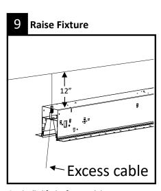
Gradually lift the first module to approximately 12 inches below the ceiling using the aircraft cables.
