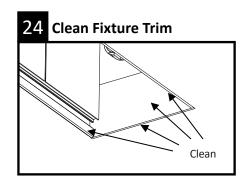
Eliminate any paint or drywall compound on inside fixture trim to ensure lens will properly insert.
