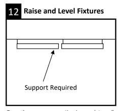
Once the power connection is complete, pull the aircraft cable to raise the first modules to just below the ceiling. Hang the next module with the far end suspended from an aircraft cable. The joining end needs to be temporarily supported for the duration of wire connections.
