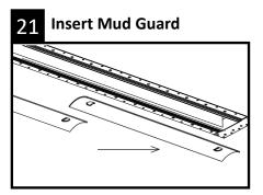
Before beginning ceiling mudding, insert the supplied mud guards into each fixture to protect fixture opening from mud and paint.
