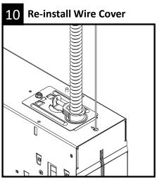
Re-install wire cover and slide to lock. Install screw.
