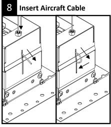
Suspend end module by inserting the aircraft cables through the grippers on top of the housing. The cable will pop out the side of the housing and should be fed back below the LED board. On the joining end, insert cable and fish it out so it hangs out of the end of the fixture.
