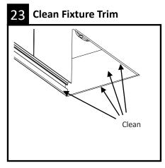
Eliminate any paint or drywall compound on inside fixture trim to ensure lens will properly insert.
