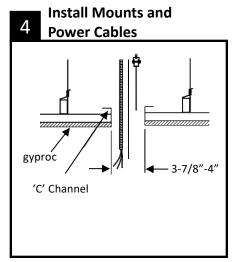
Install a 'C' channel perimeter around the ceiling cutout.
