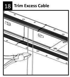
Trim suspension cable approximately 8 inches below the ceiling level. Tuck all excess cable inside the upper wiring cavity.
