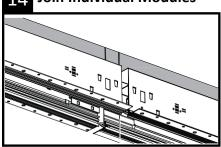
Gently slide housing modules together, ensuring joiner aligners are engaged inside the trim in the adjacent module.
