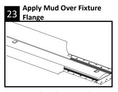
Mud over the fixture flange. When finished, use a utility knife to cut out the mud guard.
