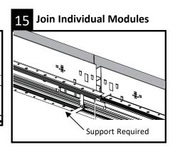
Gently slide housing modules together, ensuring joiner aligners are engaged inside the trim in the adjacent module.
