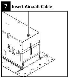
Suspend each module by inserting the aircraft cables through the grippers on top of the housing.
