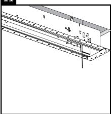
Once the power connections are complete, pull the aircraft cable to raise all modules to just below the ceiling.
