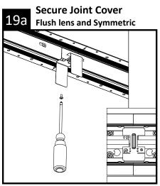
At joint location(s), secure joint covers using Philips screwdriver and supplied hardware. Ensure cover plates sit flush with bottom reflectors for proper LED board fit.
