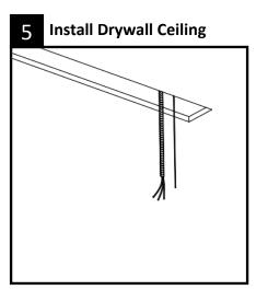
Install drywall ceiling and cut required opening as shown in **figure A** on page 2 or **figure B** on page 3.
