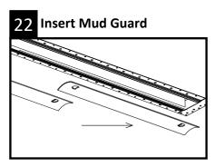
Before beginning ceiling mudding, insert the supplied mud guards into each fixture to protect fixture opening from mud and paint.
