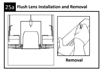
**Flush Lens:** Snap in lens into fixture. Lens Removal: To remove snap-in lens for maintenance purposes, insert a flat, smooth edged object between lens and housing. Twist to release pressure and remove lens.
