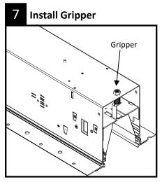
Insert supplied gripper (from joiner kit) into housing. Gently tighten gripper nut. Align gripper release key with slot on reflector pan. The first module in a run should have a gripper at each end, and all subsequent modules should have one at the end away from the previous module.
