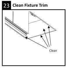
Eliminate any paint or drywall compound on inside fixture trim to ensure lens will properly insert.
