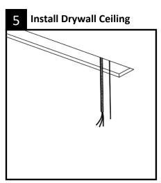
Install drywall ceiling and cut required opening as shown in **figure A** on page 2 or **figure B** on page 3.
