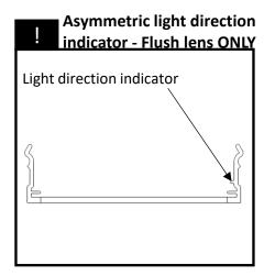
Note the knob on the inside of the lens. The asymmetric film directs to light in the direction of the knob. Always install in the fixture in the direction shown on the layout drawings.
