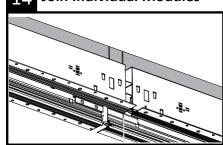
Gently slide housing modules together, ensuring joiner aligners are engaged inside the trim in the adjacent module.
