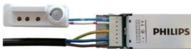
Two-wire sensor connected to driver SR interface
