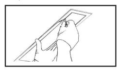
To remove snap-in lens for maintenance purposes, insert a flat, smooth edged object between lens and housing. Twist to release pressure and remove lens.
