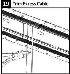
Trim suspension cable approximately 9 inches below the ceiling level. Tuck all excess cable inside the upper wiring cavity.
