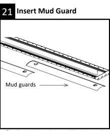
Before beginning ceiling mudding, insert the supplied mud guards into each fixture to protect fixture opening from mud and paint.
