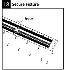
Secure the fixture to the gyproc and 'C' channel with #6 drywall screws (supplied by others). Use spacing tool every 2' to ensure the correct width of housing opening while securing the fixture to gyproc. (Spacing tool is attached to the outside of each housing.)
