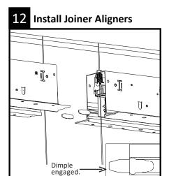
At joint location(s), gently tap provided joiner aligners inside one module only. Two joiner aligners are required for each joint. Important: To insert aligners, tap gently with a hammer until half is inserted into the joiner channel. Be sure to engage the dimple as shown.
