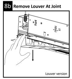
To remove louver at a joint, gently pull louver down from open end.
