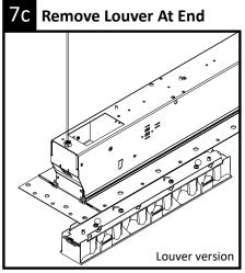
Temporarily use tape to suspend louver just below fixture. <u>DO NOT ALLOW LOUVER TO HANG FROM ELECTRICAL WIRES.</u>
