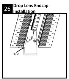
Push up drop lens endcap flush to bottom of trim while **hand tightening** with supplied screws.(8-18 x 3/8 Pan)
