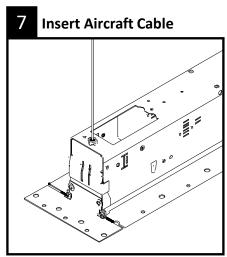
Suspend each module by inserting the aircraft cables through the grippers on top of the housing.
