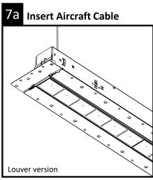
Before continuing, louvers at fixture ends need to be temporarily removed for suspension cable and gripper access.
