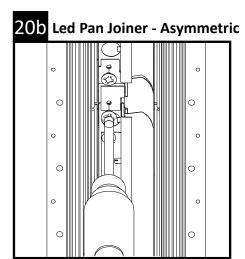
Mount the LED pan connector with the supplied screw in the joiner kit.
