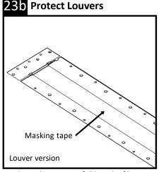
Apply masking tape to full length of louver run. Ensure all louver surfaces are fully covered.
