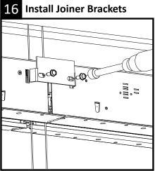
Install joiner brackets on each side of the housing using supplied hardware.
