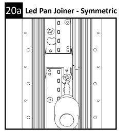
Mount the LED pan connector with the supplied screw in the joiner kit.
