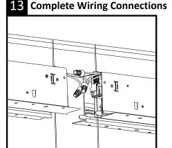
Complete module to module wiring connections and carefully tuck all wires inside the upper wiring cavity.
