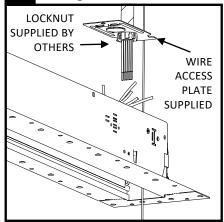
At power location(s), feed power wires through supplied wire access plate. Complete all wiring connections using wire nuts supplied by others.
