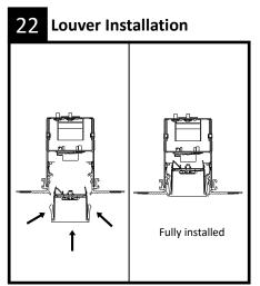
Install louvers previously removed for installation.
