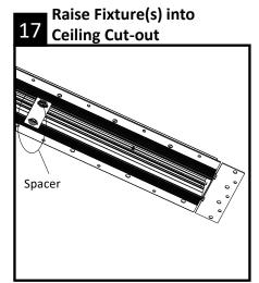
Important: For continuous row modules, start at one end and gradually raise each module up one inch at a time. Repeat process until housing is fully recessed and housing trim touches drywall ceiling. Do not stress the joint connection by tilting the module, as damage can occur.
