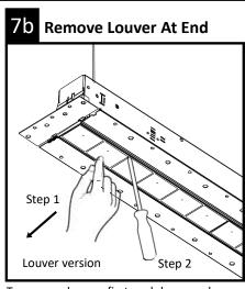
To remove louver, first push louver edge away with one hand, then gently pry opposite side with a thin, flat screwdriver.
