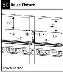
Temporarily use tape to suspend louver just below fixture. <u>DO NOT ALLOW LOUVER TO HANG FROM ELECTRICAL WIRES.</u>
