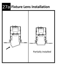
Snap in lens into fixture.
