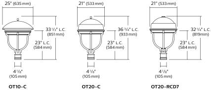
EPA: 1.74 sq.ft. Weight: 40.5 lbs. (18 kg) EPA: 1.42 sq.ft. Weight: 40.5 lbs. (18 kg) EPA: 1.42 sq.ft. Weight: 40.5 lbs. (18 kg)
