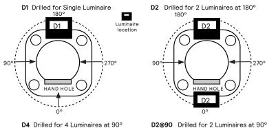
D2 Drilled for 2 Luminaires at 180° 180° D2 2709
