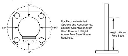
Orientation is measured clockwise from the Hand Hole Center.
