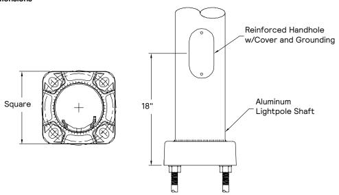
**NOTE**: Factory supplied template must be used when setting anchor bolts. Gardco will not honor any claim for incorrect anchorage placement from failure to use factory supplied templates.
