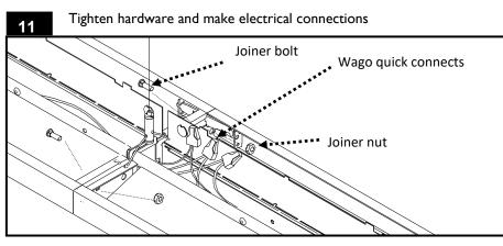
Ensure both fixtures are horizontal and suspended at the same height. Snug jointing nuts using 3/8" nut driver, align the fixture housings for best aesthetic before final tightening. Complete necessary electrical connections in compliance with local codes. Close all wire access panels (step 7) when complete.
