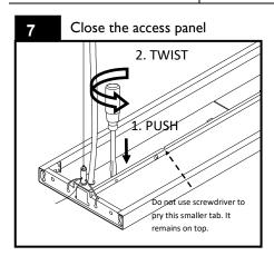
Ensure the electrical connectors are tucked inside the wire cavity. Push down on the lid while simultaneously twisting the flat blade screwdriver, the panel tab will lock into place. Repeat at the other screwdriver slot location. For standalone fixtures skip ahead to step 12.
