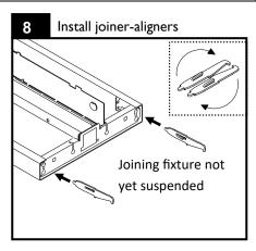
Prepare the joining fixture by twisting apart the joiner pair and inserting into crossplate (DO NOT INSERT INTO THE FIXTURE ALREADY SUSPENDED). Open the wire access panel of the joining fixture.
