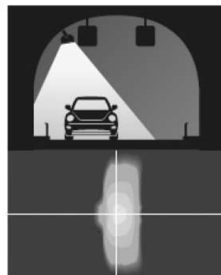
Typical 2 lane narrow tunnel / cornice configuration
