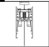
Insert aircraft cable into the gripper. Repeat on the other end of the fixture. Raise module 1 towards ceiling, suspending both ends a few inches below ceiling level.
