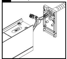
For surface mounted junction box, connect conduit and required connectors (by others) to drilled endcap. Refer to 9a & 9b.
