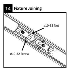
Secure fixture modules together using the two #10-32 machine screws and the two #10-32 nuts supplied. Tighten until joint seam is tight. **Note:** Do not overtighten.
