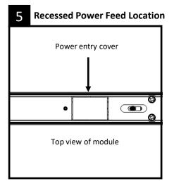
Determine fixture power feed method and location. For a recessed utility box installation, break off power cover tabs using a flat screwdriver at required end only. Power entry location available only on one side on module lengths 2',2.5'3' and 3.5'.
