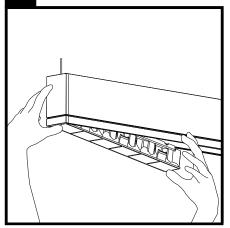
Reinstall surface plates with the screws provided and follow with louvers. Start on one end of the louver pressing gently on side tabs. **IMPORTANT:** For asymmetric louver fixtures, orientate the arrows on the louver pan to point at the label on the outside of the housing.
