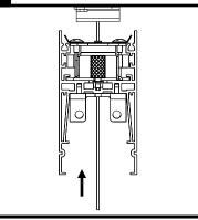
Raise the row of modules to ceiling simultaneously. Tighten join again if required. Now the whole row is secured. Push excess aircraft cable through the opening.
