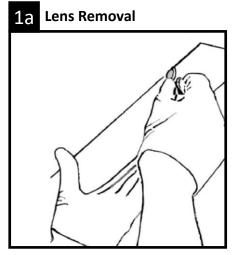
Lens Removal: To remove snap-in lens for maintenance purposes, insert a flat, smooth edged object between lens and housing (avoid screwdrivers). Twist to release pressure and remove lens. Note: Optional Drop Lens is shipped separately.
