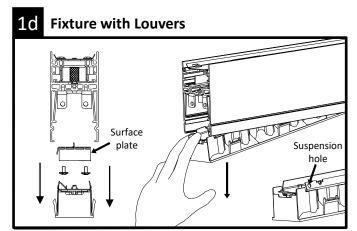
Remove one louver from end of fixture by pulling gently and temporarily suspend from available holes. Remaining louvers can be pushed to center for better access. Remove the screws securing the surface plate. For louver-lens combinations, remove both louver and lens. Use cotton gloves to handle lenses and keep in a clean environment.
