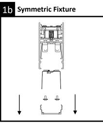
Remove lens from fixture and set aside until fixture installation is complete. Use cotton gloves to handle lenses and keep in a clean environment. Remove the 2 screws securing the lower light engine and temporarily support light engine in position below fixture.
