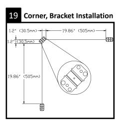
If a corner is required, it is recommended the corner module be installed first. Position of brackets are critical for installation. Place as dimensioned above.
