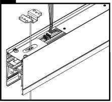
While supporting the module in the air complete power entry wiring connections. Ensure all connections are secure and all wires are neatly tucked inside fixture wiring cavity.
