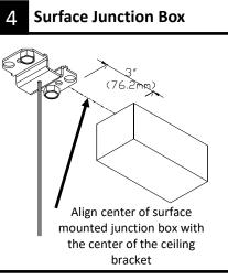
For a surface mounted junction box, install junction box as required. For a cleaner install and better alignment with installed fixture modules, center junction box and conduit exit with center line of ceiling brackets. Junction box is required to be 3" (minimum) away from mounting bracket.
