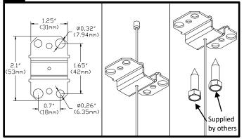
Determine location of ceiling brackets. Pull aircraft cable thru the bracket. Center and install ceiling brackets to structure (studs or cross-braces) using appropriate hardware (by others).
