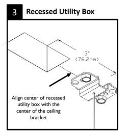
For a recessed 2"X4" utility box, align and center with ceiling brackets, and install with long edge parallel with fixture module length. Ensure utility box is positioned 3"(center to center) away from ceiling bracket.
