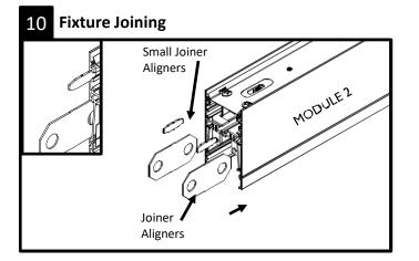
With module 2 on the ground, tap small joiner aligners inside top chase. Ensure small joiner aligners are inserted more than halfway inside fixture housing. Insert large joiner aligners inside lower chase as shown.
