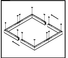
If installing a square or rectangular closed pattern, it is recommended to install opposite U-shaped fixture/corner patterns first and complete the installation by bringing U-shaped sections together as shown.
