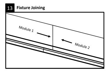
Ensure all connections are secure and all wires are neatly tucked inside fixture wiring cavity. Slide fixture modules together gently.
