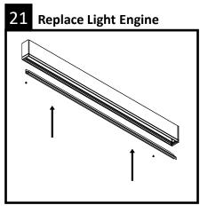
Reinstall the lower led pans with the screws provided. Ensure direction of light is as shown on layout drawings.
