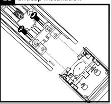
Slide endcap onto end of fixture module and secure from below using two #8-32 X 3/18" screws. Tighten screws until endcap seam is tight. Note: Do not overtighten.
