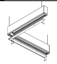
Reinstall the surface corner plates with the screws provided.
