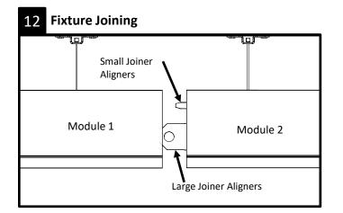
Bring module 1 and 2 together. Engage joiner aligners in module 2 with housing of module 1.
