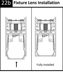
Once lens is positioned inside housing, starting on one end or joint, push upwards gently and work outward to complete the run.
