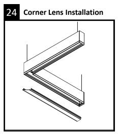
Installation Tip: For easier installation of corner lenses, start at the corner and work outward to complete the run. Follow step 22.
