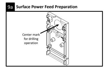
For surface junction box installation, power feed to fixture module is done through the endcap. Use masking tape on all outside surfaces. Align with center mark as shown and drill a 7/8" diameter hole.
