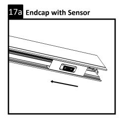
Before installing the endcap, slide the sensor towards the center of the fixture to gain access. Proceed with endcap installation, step 18.
