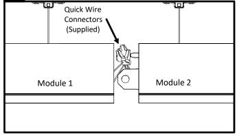
Suspend Module 2. Refer to step 7. With module 2 supported complete wiring connection using provided quick wire connectors. Note: Do not fully raise modules at the moment.
