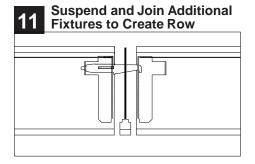
Raise next fixture to cantilever bracket and insert the joiner aligners into the corresponding slots on the already installed fixture.
