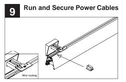
Run power cable down fixture channel and through power plate at the end of the fixture. Secure power cable into fixture channel using supplied cable clips at 4 increments.
