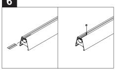
On the floor, slide power plates into fixture ends. Attach supplied bushings in power locations and plugs in non-power locations.
