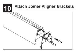
On the floor, slide variable mount bracket into next fixture in run. Attach joiner-aligner brackets into opposite side.
