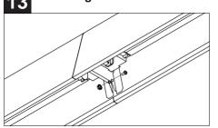
Join fixtures using supplied #8 screws and lock-nuts. Repeat steps 8-12 for each fixture in run.
