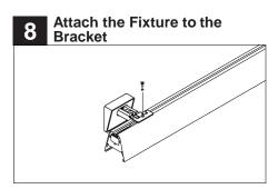
Raise fixture to brackets and use the supplied countersunk screw with countersunk washer to attach the fixture to the bracket. Adjust fixture hanging brackets so fixture is flush with cantilever arm and tighten.
