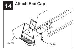
Snap on the gasket to the end of the fixture and attach end caps using supplied #8 screws.
