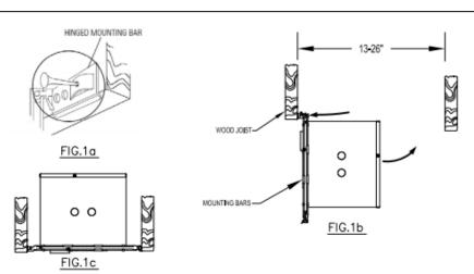
NOTE: To insure proper installation it is important the mounting frame always be secured to structural ceiling members
