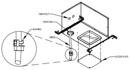
CAUTION: To reduce risk of electric shock wires must be capped and not energized.
