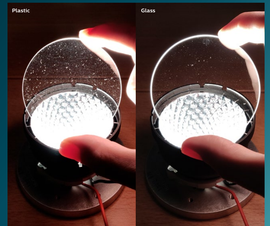
Figure 11: A comparison of dust and scratches on plastic and glass front covers, which were both cleaned with a microfiber cloth before the photo was taken
