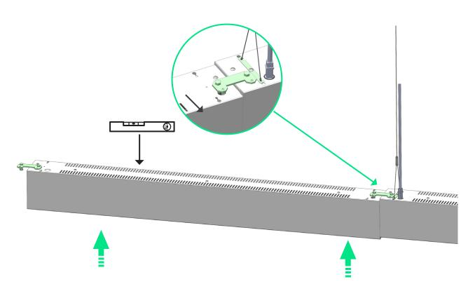
Secure trunking plate by tightening bolt and secure other end of supsension cable with saftey bracket
