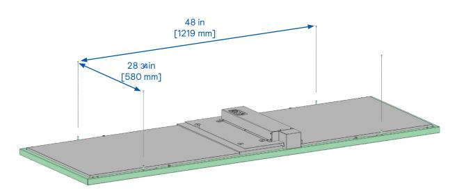
Check mounting instruction for suspension points installation (4).
