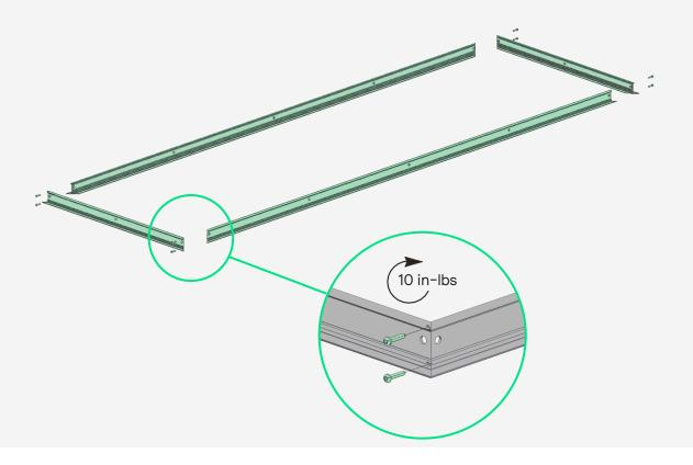
Mount frame to ceiling and then luminaire to frame
