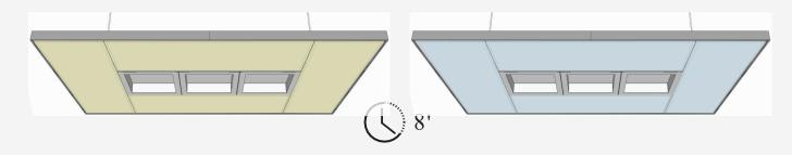
If any of the Daylight remains static, please check if all cables are connected correctly.
