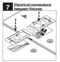
Feed the wires through the nipple and make all the electrical connections between the fixtures following the correct wiring color code. Attach the wiring access cover plates.
