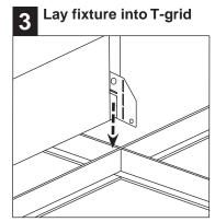
Lay fixture into T-grid.
