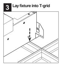
Lay fixture into T-grid.
