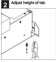
Use side cutters to adjust each tab to he height of the T-bar.
