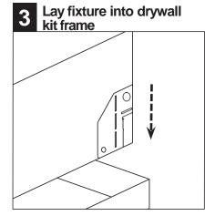
Lay fixture into drywall kit frame.
