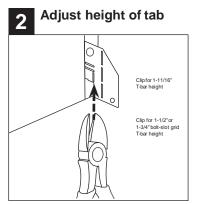
Use side cutters to adjust each tabto height of T-grid.
