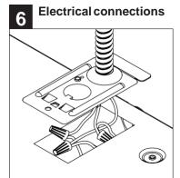
Make all electrical connections to the fixture.
