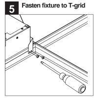
Use a #8x1/4 sheet metal screw to fasten fixture to the T-bar grid and use a hanger wireto tie off appropriately in accordance with local building codes (screws and hanger wires supplied by others).
