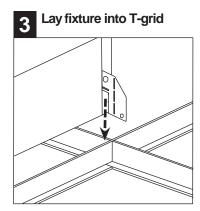
Lay fixture into T-grid grid.
