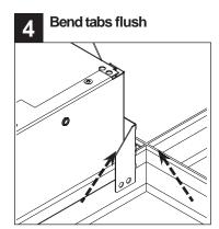
Bend tabs flush against the T-bar in order to clear the ceiling tile.
