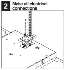
Make all electrical connections to the fixture. Attach wire access cover plate.
