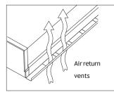
The air return version features slotted vents along the sides of the fixture. As a result, the installation method of the air return version is different to the standard version, and the fixture cannot be installed in continuous
