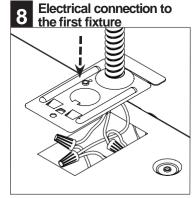
Ensure that the wiring of the last fixture in the row is properly terminated. Then make all electrical connections to the first fixture in the row. Attach the wiring access cover plate.
