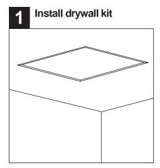
Install drywall kit frame in ceiling. Refer to Drywall Kit specification sheet for mounting options and ceiling opening sizes.
