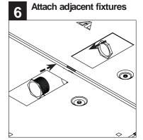
Remove connecting knock-outs and attach adjacent fixtures to the T-grid following steps 1-5. Place a 1/2" nipple through the knock-out hole between the fixtures. Fasten with a 1/2" NPT lock nut (nipple and lock nut supplied by others).
