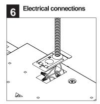
Make all electrical connections to the fixture.
