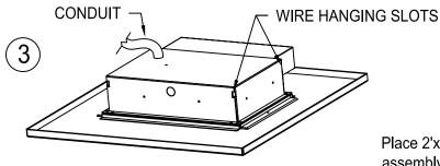
Place 2'x2' faceplate and enclosure assembly into ceiling grid. Connect AC service conduit to enclosure. Rectangular slots are provided at each corner of enclosure for wire hanging as shown.
