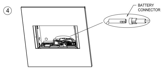
Connect red battery lead by pushing connector halves together (see above). Make AC service connections. See table below for wiring guide.
