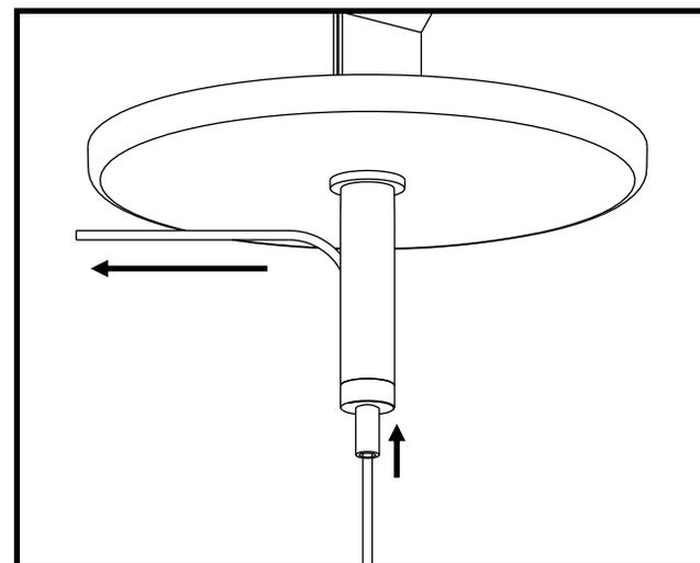
POUR DÉGAGER LE CÂBLE D'AÉRONEF, POUSSER SUR LA PETITE TIGE DANS LA PARTIE INFÉRIEURE DU DISPOSITIF DE RÉGLAGE.
