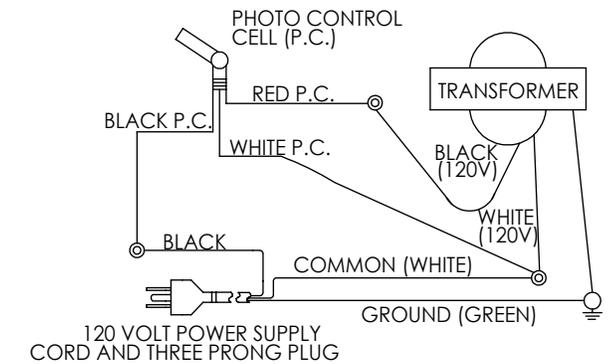
WIRING AFTER PHOTO CONTROL INSTALLATION
