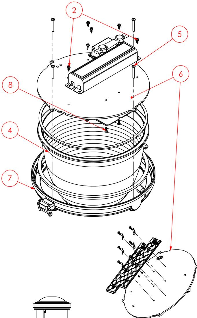
**Release the latch to open the luminaire.**
