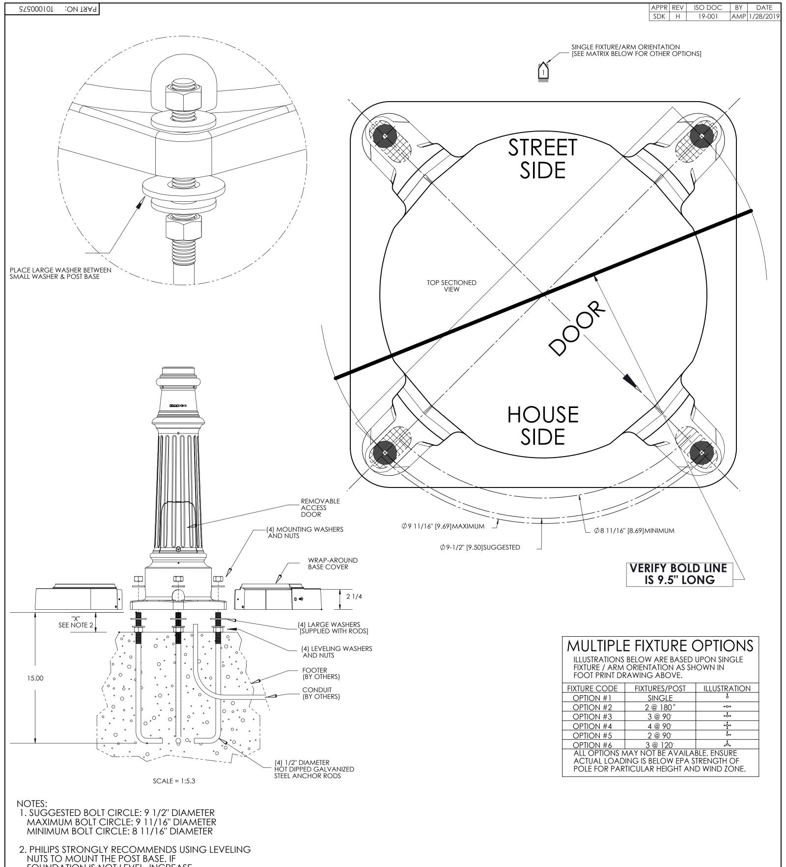
2. PHILIPS STRONGLY RECOMMENDS USING LEVELING NUTS TO MOUNT THE POST BASE. IF FOUNDATION IS NOT LEVEL, INCREASE "X" DIMENSION ACCORDINGLY WHEN USING LEVELING NUTS WITH WASHERS.
