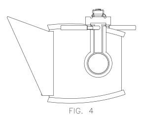
VISOR MAY ALSO BE INSTALLED IN THIS ORIENTATION
