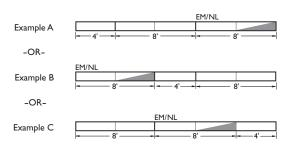
IMPORTANT: Whenever longer rows are made up of both 4' and 8' modules, EM/NL/BP\* sections will always be installed in 8' modules. If specific site restrictions require EM/NL/BP\* sections to be installed in 4' sections. please contact the factory.
