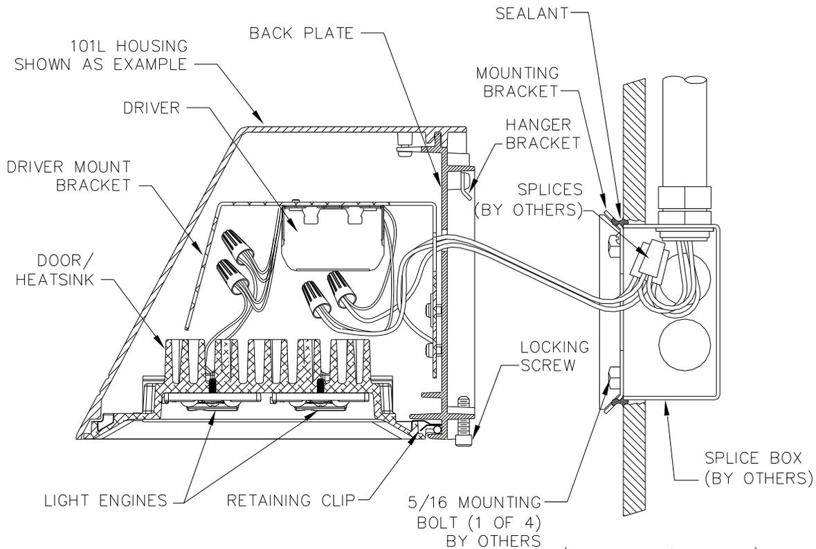
1. APPLY A BEAD OF SEALANT ON WALL AROUND SPLICE BOX OPENING AND AROUND HOLES USED FOR OPTIONAL MOUNTING BOLTS OR SCREWS. WHEN USING A 4" OCTAGONAL BOX (SHOWN), FILL GAP BETWEEN WALL OPENING AND SPLICE BOX WITH SEALANT.
