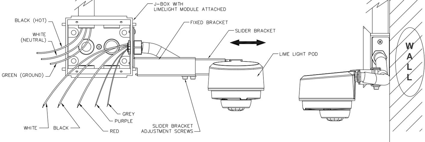
**INSTALL / MOUNT THE LIME LIGHT MODULE WITH J-BOX TO THE WALL / SURFACE USING (4) 5/16 BOLTS SUPPLIED BY OTHERS.**
