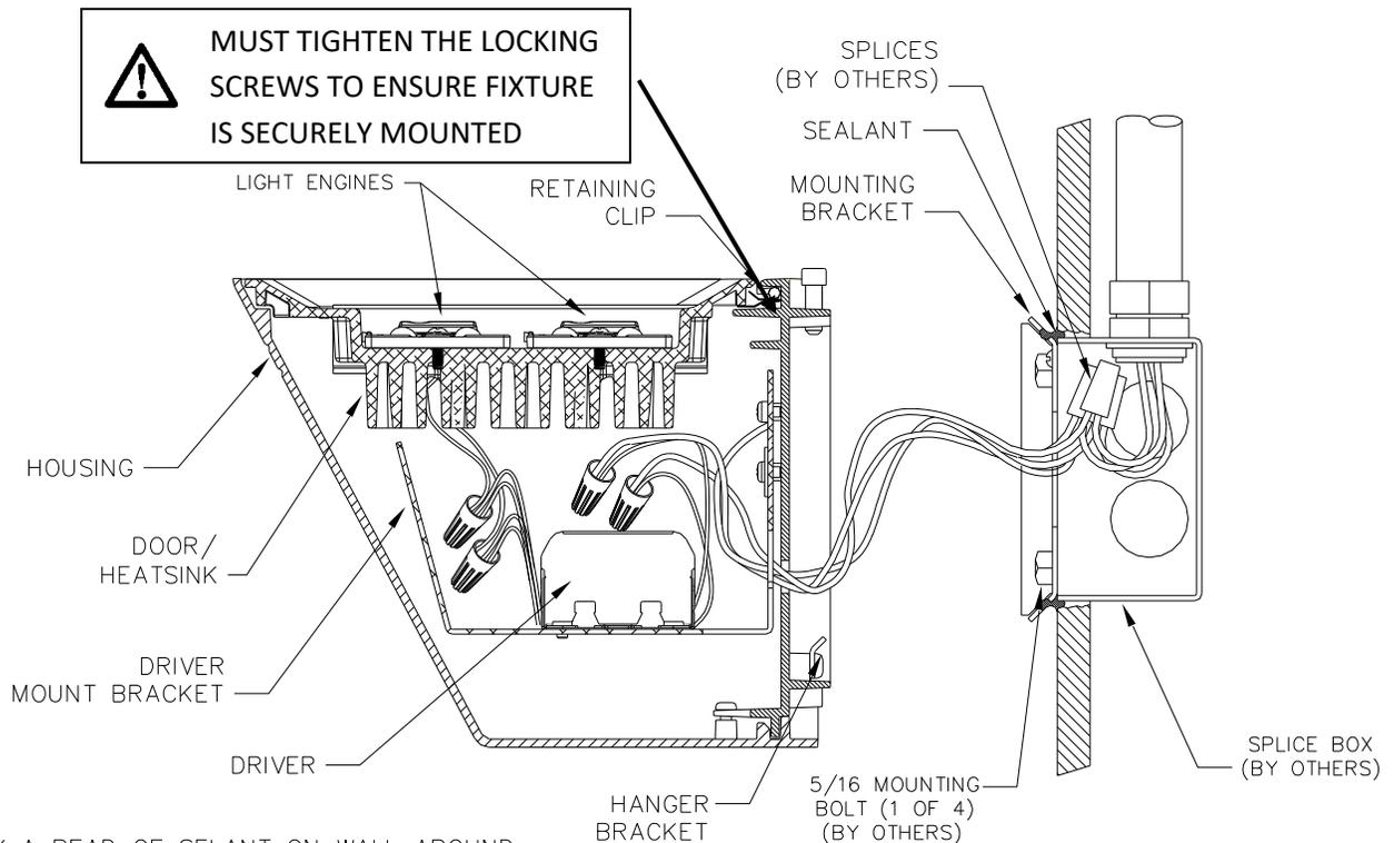
1. APPLY A BEAD OF SELANT ON WALL AROUND SPLICE BOX OPENING AND AROUND HOLES USED FOR OPTIONAL MOUNTING BOLTS OR SCREWS. WHEN USING A 4" OCTAGONAL BOX (SHOWN), FILL GAP BETWEEN WALL OPENING AND SPLICE BOX WITH SEALANT.
