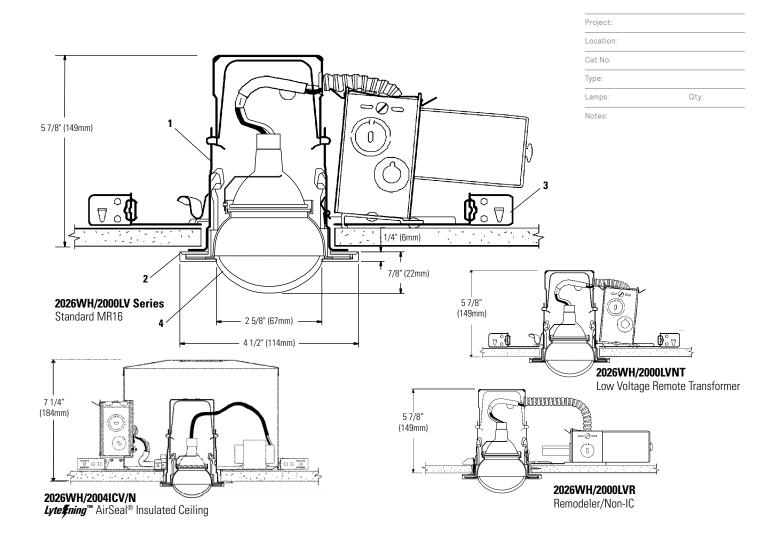
Complete Fixture consists of Reflector Trim & Frame-In Kit. Select each separately.
