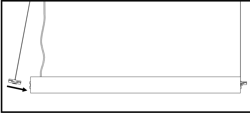
Slide joiner bracket into power entry side of the luminaire.
