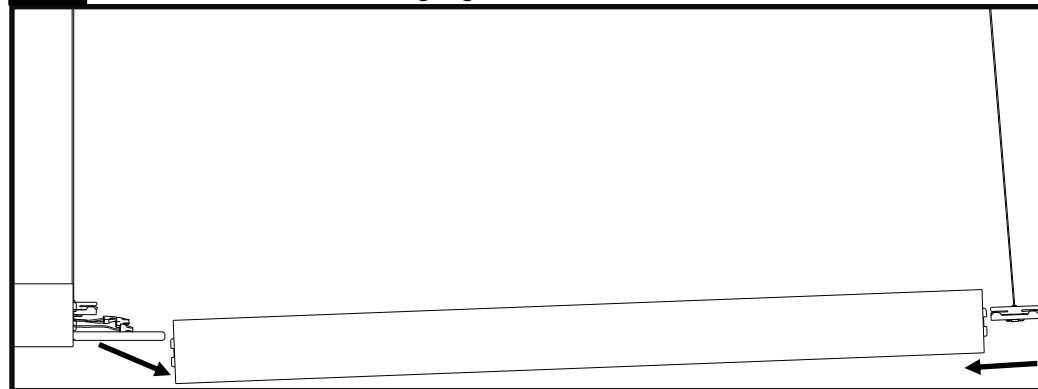
Slide joiner bracket into far side of the next luminaire in the row. Ensure that the bracket is fully seated and clicks into place. Slide luminaire onto aligner brackets of the previous luminaire.
