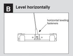
LEVEL HORIZONTALLY (shown above): Loosen fasteners on bottom of adjuster and level as required. Tighten fastener once fixture is in level position.
