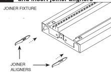
For each additional fixture in the row, at the end furthest from the existing suspended fixture, attach A/C mounting bracket to fixture using supplied fasteners (see step 2). At the end closest to the existing suspended fixture, insert joiner aligners into crossplate (aligners will lock into place).
