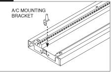
A. Hook A/C mounting bracket to endplate as shown. Raise bracket until security tab is engaged.
