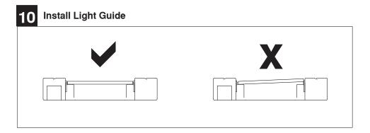
Identify smooth side of the Light Guide and ensure it is installed smooth side DOWN. Install Light Guide panel into LED fixture after joining and wiring is complete. Ensure panel is seated correctly as shown above.
