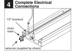
NON-POWER LOCATIONS: Cap all wires and tuck into wire cavity.
