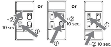
If the switch joins the group then the luminaire will FLASH twice and group light level will go to 5%.
