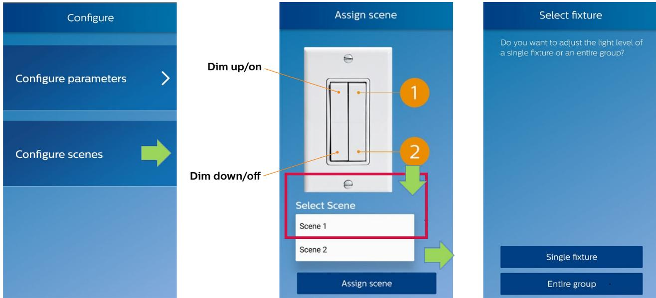
The scenes are selectable via the scene buttons of the switches associated either to fixture or an entire group. In any case, the configuration proceeds through the "Adjust light level" screen that enables the user to select desired light level for the selected scene.
