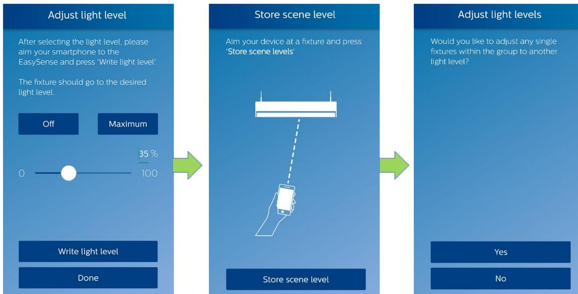
For a given scene, individual fixtures within the group can be configured to different light level settings. This is beneficial for example in a conference room where fixtures closer to the projection wall are desired to be dimmed/off while other fixtures in the same group are desired to be at higher light levels on the same scene.
