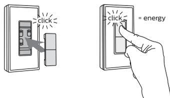
All the luminaires in the group will turn on/off based on the rocker pad action.
