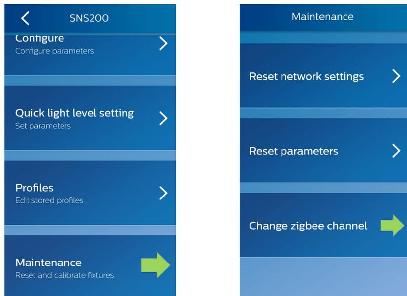
**Note:** If Zigbee channel is changed on the luminaires, then any switches part of the group will have to be re-joined to the group because the switches do not change their Zigbee channel and rejoining action will ensure that the switches are operating on the same new channel as the luminaires.
