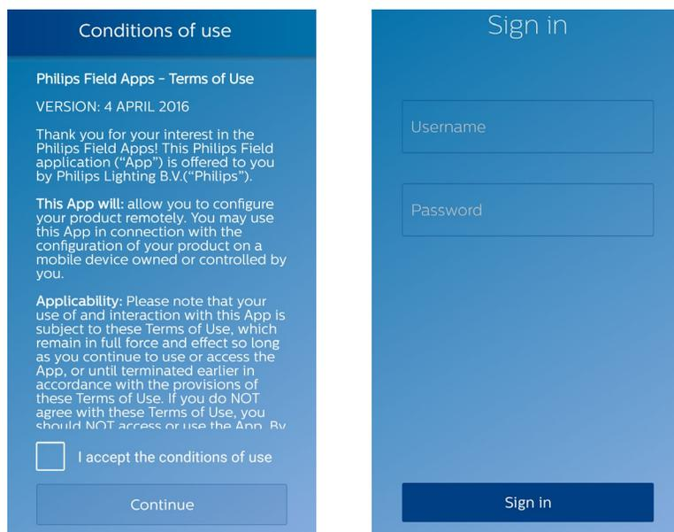
There are two application modes within the Philips Field App for configuring EasySense and SpaceWise DT. These modes are EasySense NFC and EasySense IR. The EasySense IR mode can be used to commission (group) luminaires and add wireless switches to the group, while the EasySense NFC mode can be used to read out sensor parameters.
