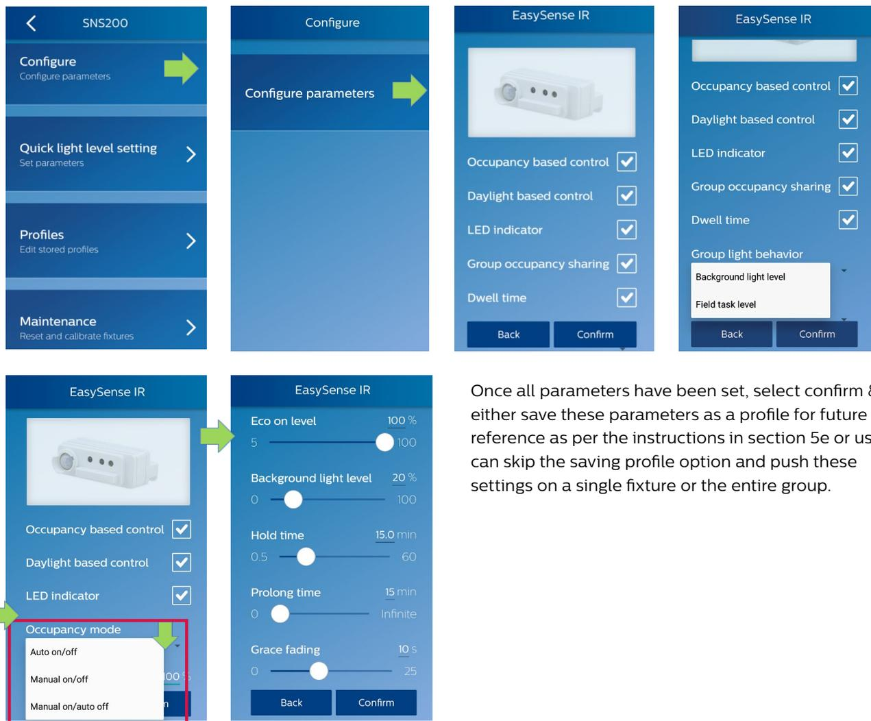
Once all parameters have been set, select confirm & either save these parameters as a profile for future reference as per the instructions in section 5e or users can skip the saving profile option and push these settings on a single fixture or the entire group.
