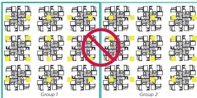
When configuring open plan offices with SpaceWise DT, large groups of 30-40 luminaires are recommended to maintain the lighting aesthetics of the space. Smaller groups may turn off more frequently than desired.
