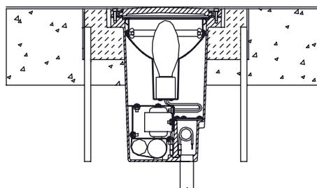
SL-33 In Concrete With Grout Mask
