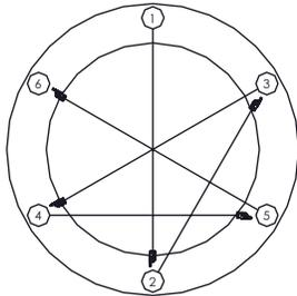
Use several rotations of the following sequence to tighten the lens ring screws, to 25 in/lbs.
