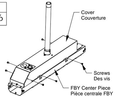
Screw the cover onto the plate at 4 locations and then screw the cover's front opening at 2 locations as shown in the diagram
