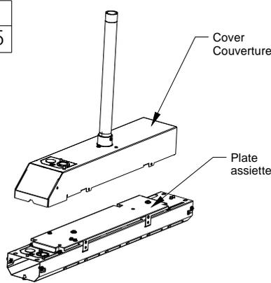
Make all the necessary electrical connections and then, snap the Cover onto the Plate by aligning 4 holes on cover and plate
