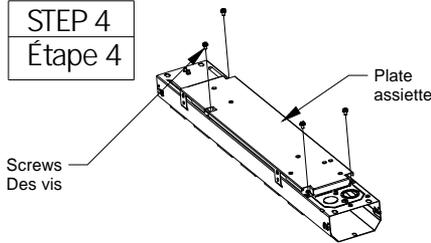
Screw the Plate to the FBY center piece in 4 locations as shown in the diagram
