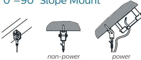
Versatile mount designed for flat or sloped non-accessible ceilings (0°–90° slope) where the electrical box is pre-installed either surface mounted or recessed in the ceiling. Exposed mounting hardware provides more industrial look.
