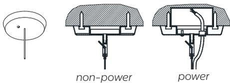
Designed for flat or gently sloping non-accessible ceilings (0°–15° slope) where the electrical box is pre-installed either surface mounted or recessed in the ceiling. System conceals mounting hardware to provide a clean, finished look.
