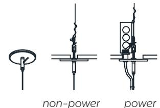
Note: Supports T-grid (15/16" and 9/16") and Slot T-grid (9/16" x 5/16") ceiling types.
