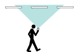
Holding the phone closer to eye level or lower will result in a wider IR range or cone. This will cause multiple luminaires to receive the signal.
