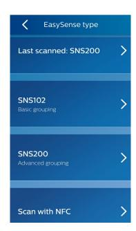
**Note 2**: Just one (any) SpaceWise DT sensor needs to be scanned, there is no need to scan multiple sensors. Once the Dwell Time feature is populated into the app, it will stay there until the phone is switched off or the app is updated or deleted.
