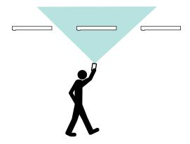
For proper commissioning, hold the phone above your head, pointed at the luminaire that you wish to target. This will help ensure that the IR range or cone is restricted to just one luminaire, and only that luminaire will react.
