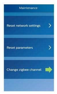
**Note:** If Zigbee channel is changed on the luminaires, then any switches part of the group will have to be re-joined to the group because the switches do not change their Zigbee channel and rejoining action will ensure that the switches are operating on the same new channel as the luminaires.
