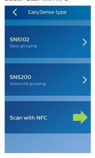
Place the back of the smartphone (where the NFC reader is located) onto the sensor NFC antenna (almost touching) to enable NFC communication. NFC communication might take a few seconds. Do not move until you hear a beep and the next screen appears.
