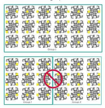
When configuring open plan offices with SpaceWise DT, large groups of 30–40 luminaires are recommended to maintain the lighting aesthetics of the space. Smaller groups may turn off more frequently than desired.
