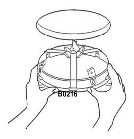
2. Slide MOUNTING CLIP down to trap ceilig thickness.
