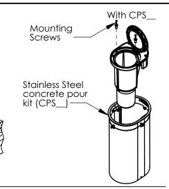
STEP 2: Connect conduit using thread sealant.
