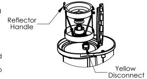
STEP 8: **NOTE:** To help decrease moisture, energize fixture for 20 minutes prior to sealing the main lens assembly. Ensure gasket seating surfaces are clean and free of debris before sealing.
