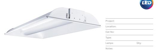
The Day-Brite / CFI HP90 LED recessed family is one of our popular soft light collection of luminaires. This is the first introduction of LED with a direct/indirect appearance utilizing highly reflective paint on the soft contoured reflectors and high light transmission linear prismatic lens to enclose the LEDs.
