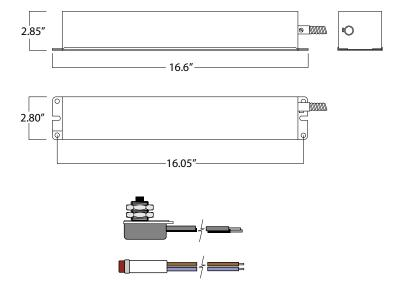
A test switch and charging indicator light is provided
