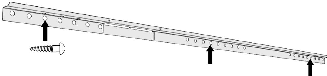
**ALIGNER, NIVELER ET RATTACHER LE RAIL MURAL SUR LA STRUCTURE AVEC UN MINIMUM DE 4 ATTACHES PAR SECTION DE 4 PI**
