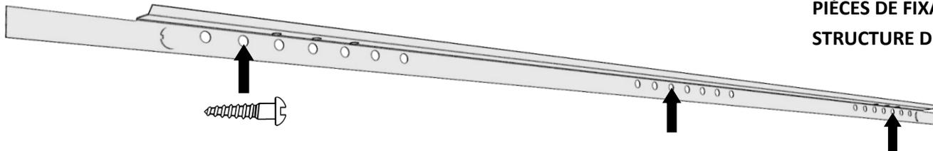
**L'INSTALLATEUR EST RESPONSABLE D'UTILISER LES PIÈCES DE FIXATION ADÉQUATES POUR LE TYPE DE STRUCTURE DERRIÈRE LE RAIL**
