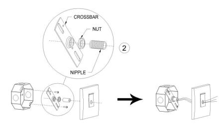
A. END AND WALL MOUNTING - Route AC supply wires thru knockout in exit housing and hang exit on nipple (end mount shown- back mount similar). Route AC supply wires thru nut and fasten to nipple to secure exit to wall. A wrench is provided in the canopy kit for this purpose.
