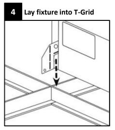
Lay fixture into T-Grid.
