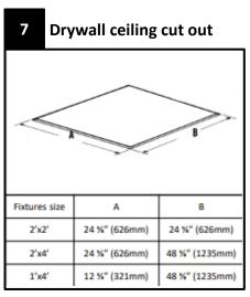
Cut a hole in the drywall according to the dimensions in the table above.
