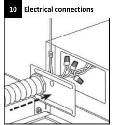
Make all electrical connections to the fixture. For flex whip option, see step 11.
