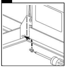
Use #8x1/4" sheet metal screws to fasten fixture to T-Grid and use a hanger wire to tie off appropriately in accordance with local building codes. (Screws and hanger wires supplied by others).
