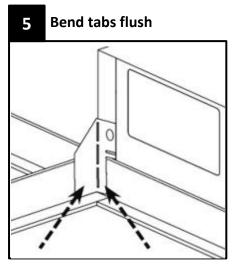
Bend tabs flush against T-Grid in order to clear for ceiling tile.
