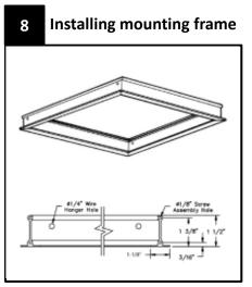
Insert mounting frame into hole and secure as showing in step 9.
